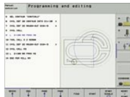
Figure 1: Traverse paths during roughing
