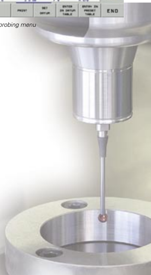
Figure 3: Probe cycle with value transfer to the preset table
