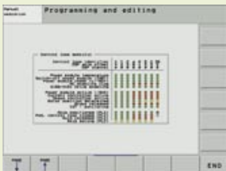
Viewing control-loop relevant information with the status LEDs on the iTNC 530 and with TNCdiag
