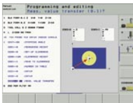
Figure 3: Probe cycle with value transfer to the preset table
