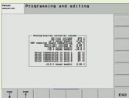
Viewing the analog signals of the drive system on the iTNC 530 and with TNCdiag
