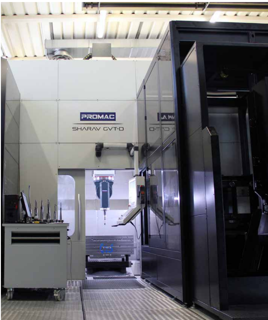
Networked: The iTNC 530 is the control center for the entire automated system.
