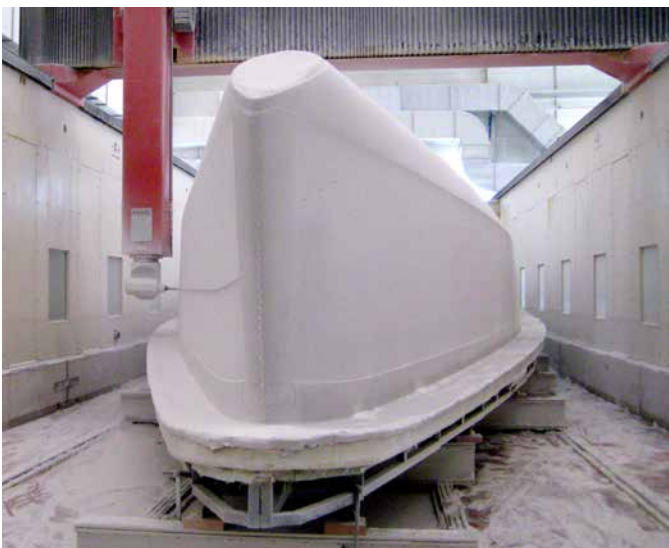
The 20.37 m long hull form with a tolerance of only 1 mm take form in the Belotti machining center.
