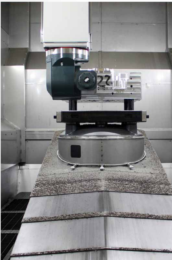
Flexible: The tilted table permits drilling and milling with five axes on five surfaces.
