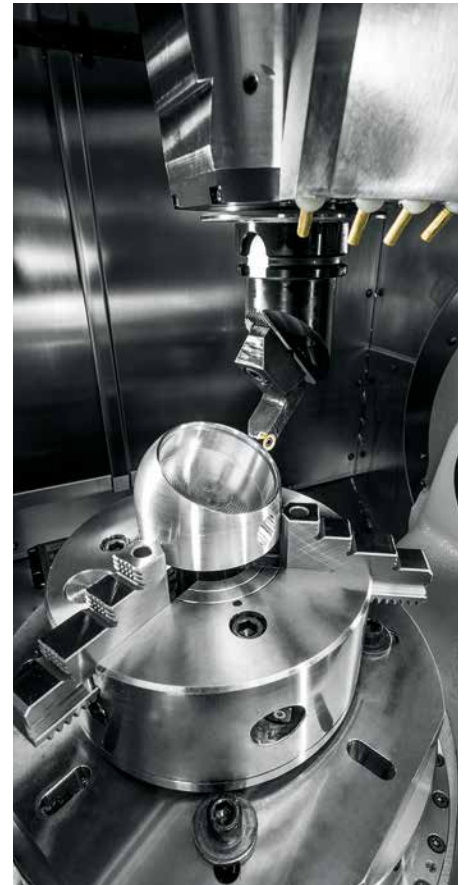
Interpolation turning: The TNC 640 enables simple and flexible machining with cycles 291 and 292—even with a tilted working plane.
