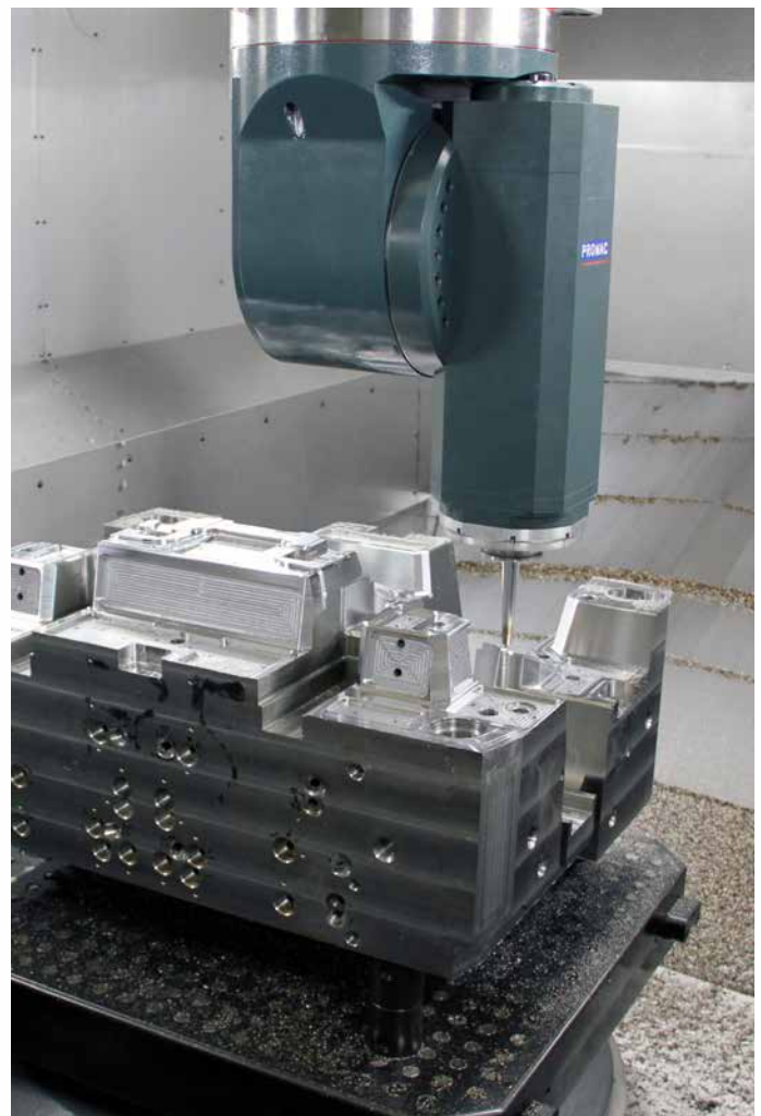
Adaptable: The machine head changing system enables all types of machining on one machine.
