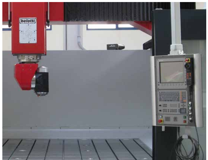
Upon Persico Marine's express wish, the Belotti machining center is controlled by a HEIDENHAIN iTNC 530.
