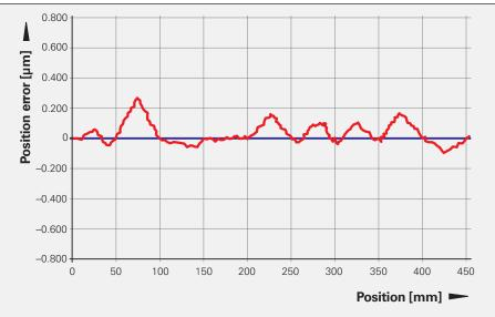
Figure 3: Residual error after multipoint linear error compensation
