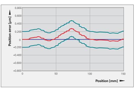
Figure 5: Total error after multipoint linear error compensation under consideration of the position error u within one signal period
