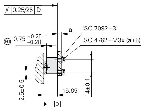
$\textcircled{H}$  = Mounting clearance between the scanning head and graduation
