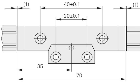
Attach the stop pins or the stop rail.
