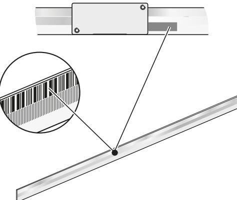
Insert the scale tape in the scale-tape carrier (do not bend it), then secure the scale tape with f xing clamp.
