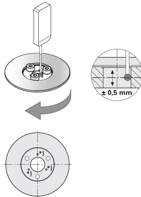
Measurement error for three-point centering
