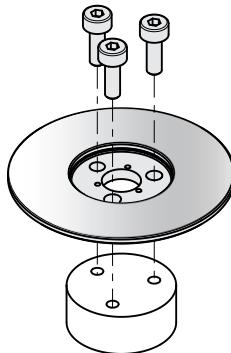
Lightly tighten the disk with hub assembly with three screws
