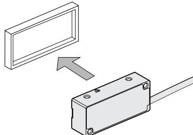
If necessary: Clean the graduation of the scale tape and scanning head with a lint-free cloth and distilled spirit or isopropyl alcohol.
