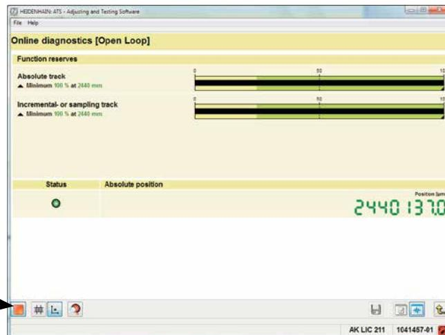
**Note:** If the green ranges are not reached or if strong signal oscillations occur over the entire measuring length, check the mounting tolerances and check for contamination.
